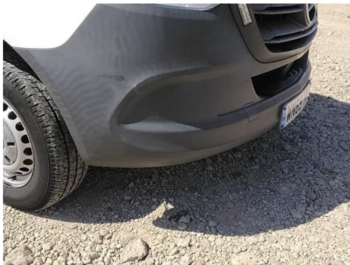
2: Bumper Front Moulding Scuffed (Unpainted) UpTo 100mm
