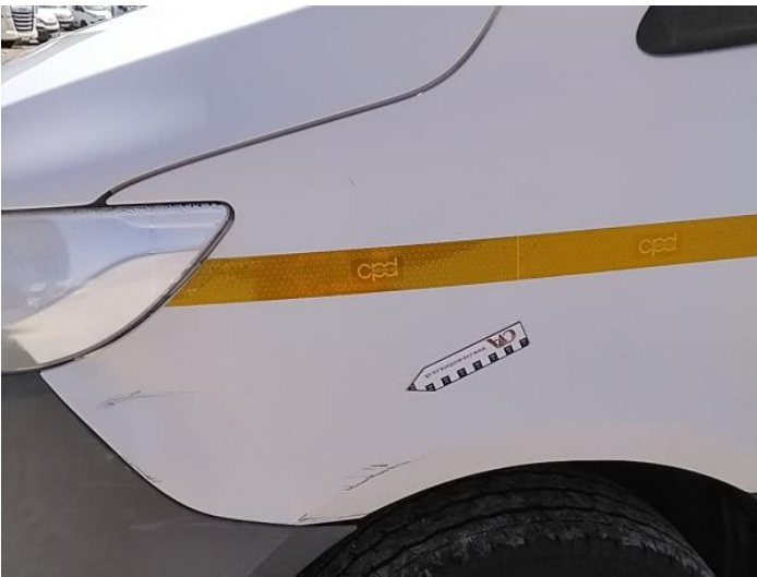
5: Wing nsf Dented With Paint Damage
