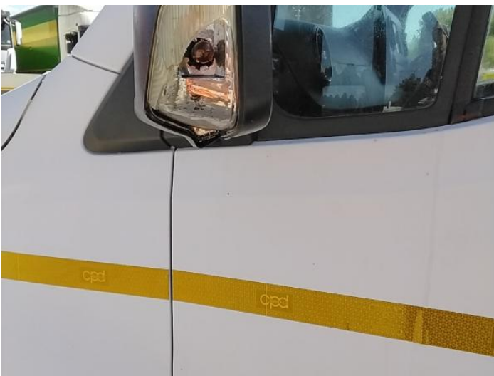
7: Flasher Side Repeater ns Broken Replace
