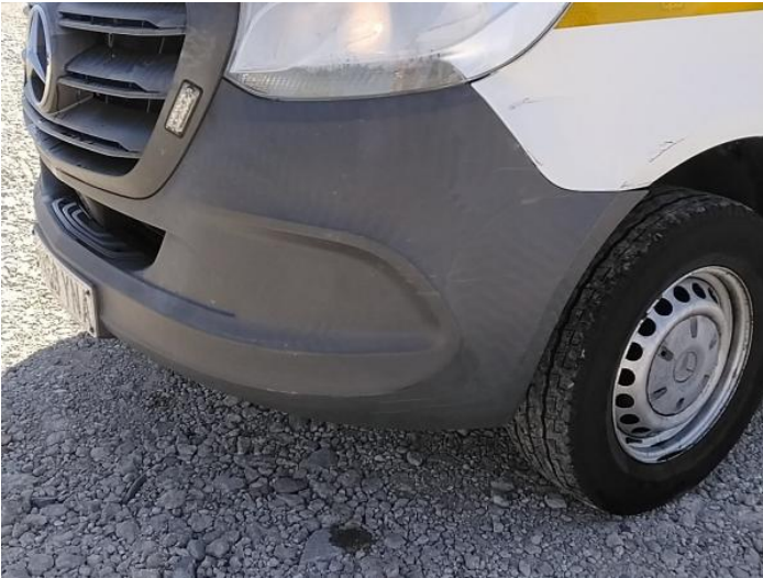
3: Bumper Front Moulding Scuffed (Unpainted) UpTo 100mm
