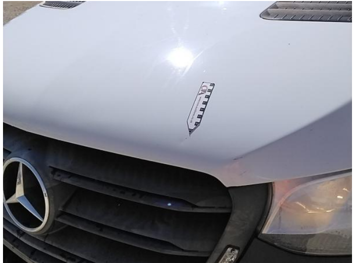
4: Bonnet Dented 2 Or Less UpTo 10mm
