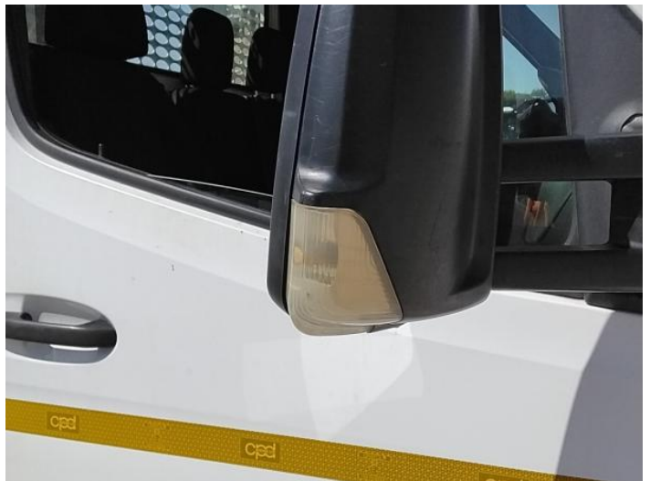
10: Door Mirror Assy osf Scuffed (Unpainted) UpTo 100mm
