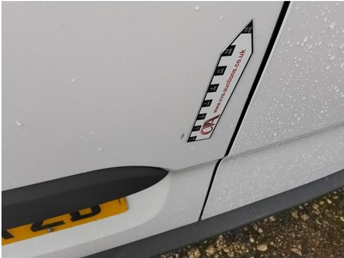
4: Door nsr Chipped Over 5mm
